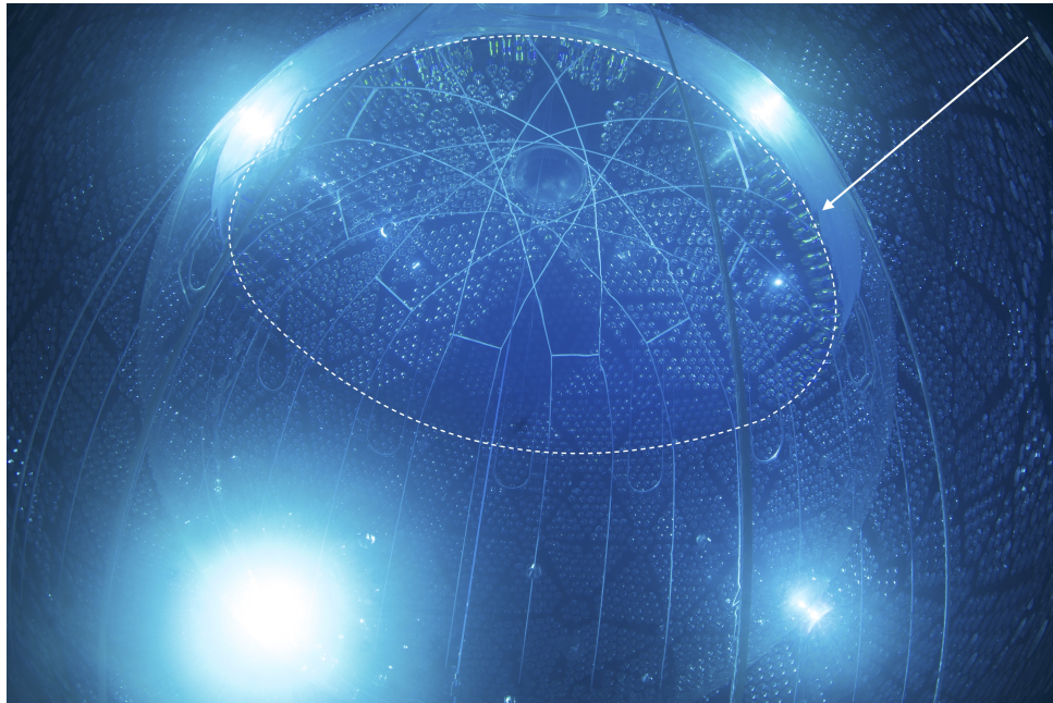
Figure 3.3: Photo of the interior of the SNO+ detector during the partial fill period. The white line and arrow highlight the scintillator–water interface.
