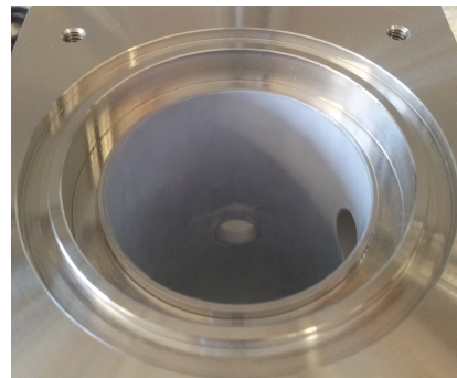
Figure 5.1.6: (a) Reflectivity spectrum of BC-622A white titanium dioxide paint. Taken from [Sai14]. (b) White paint on the inside of the aluminium cuvette. The filling hole and one hole for one of the thermometers is visible on the right.
