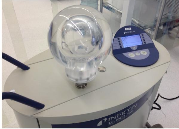
Figure 4.16: Helium-leak checking of the decay chamber using INFICON UL1000 in the LBNL clean room.
