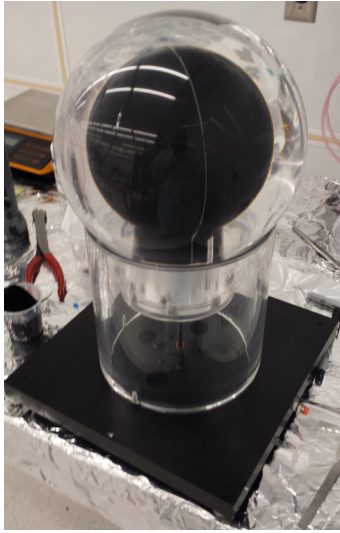
(a) Test source drying on the drying stand.
