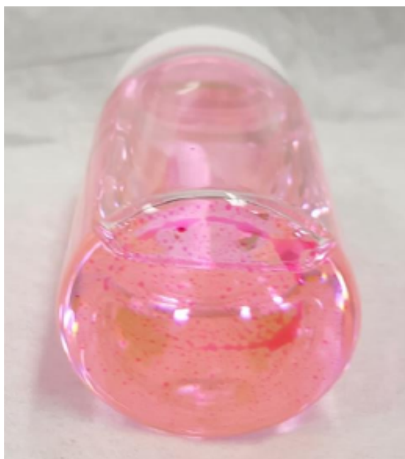
Figure 5.3: A crashed sample of TeBD in LAB, caused by titration with dyed BD.
