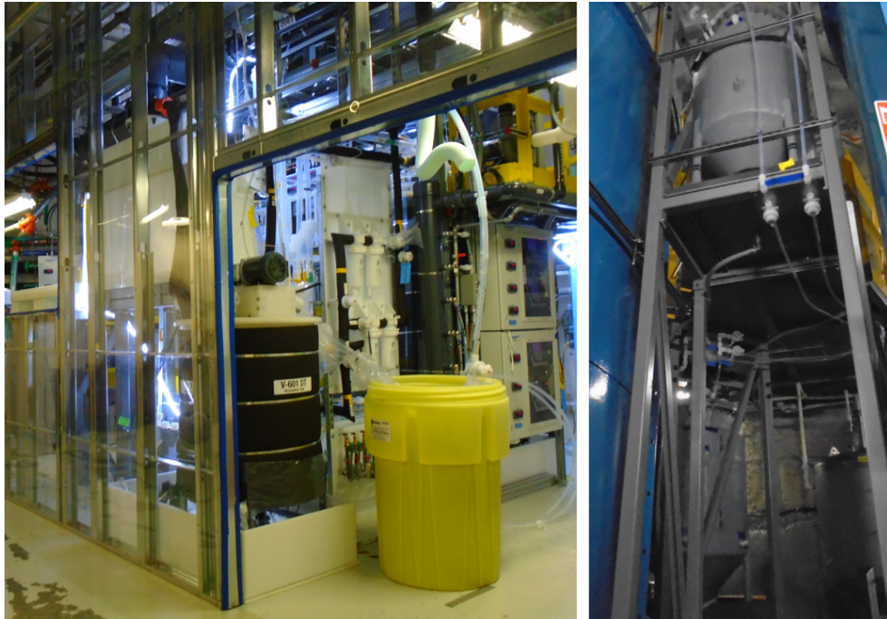
Figure 5.9: Photographs of (left) the TeA purification plant and (right) the TeBD synthesis plant.
