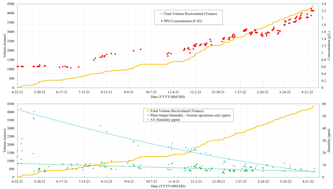
Figure 4.11: A summary of the recirculation and PPO top-up period showing (top) the addition of PPO within the detector, and (bottom) the removal of dissolved water from the AV scintillator.
