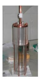
**Figure 6.42:** Acrylic vessel, or *bucket source*, with a hollow space of  $\sim 11$  for liquid scintillator. The vessel was build for deployment in the water–filled SNO(+) detector to test optical properties of LAB scintillator. The picture is taken from [248].
