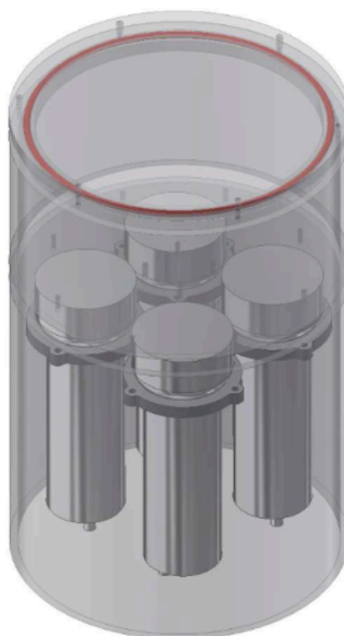
Figure 5-11: Rendering of SCOUT, showing the PMTs and scintillator volume encased in copper and lead shielding. Figure adapted from Reference [58].
