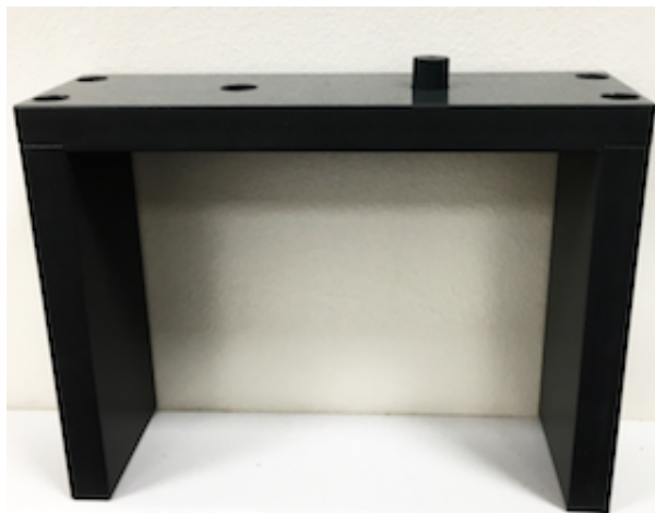
Figure 7.13: A plastic stand to support the capillary at the time of injection of an ^{90}\text{Y} droplet. A plastic holder is positioned to illustrate where a capillary is placed during the procedure.
