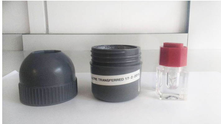
Figure 7.11: A vial for an ^{90}\text{Y} source. In the picture the vial is filled with water for training purpose. A vial with radioactive source is never taken outside of the container.
