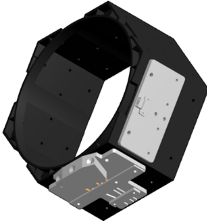
Figure 2.10: A diagram showing the mounting plates for optical fibres on the side of a PMT bucket. Figure from [73].
