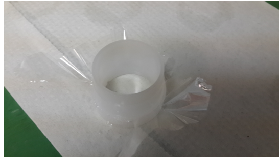
Figure 6.3: Picture of the fully assembled sample cup. New cups are used for every sample to avoid contamination.
