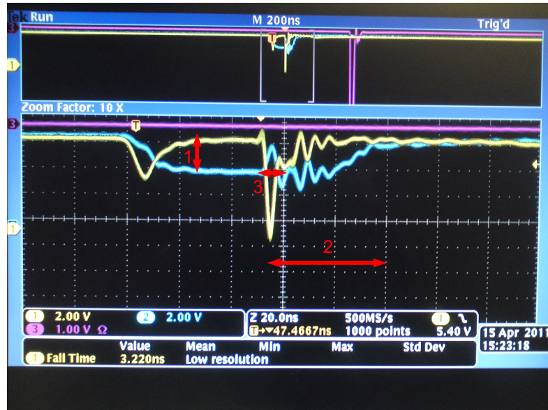
Figure 5.14: The voltages as measured at the anode (blue) and cathode (yellow) of the LED, the ringing is due to impedance miss matches at the probes. I_{OP} sets the maximum bias applied to LED (1); The Bias current I_{BI} sets the maximum length of time that the voltages at the anode and cathode of the LED can be inverted (2); I_{PW} sets the time that the voltages are inverted(3).
