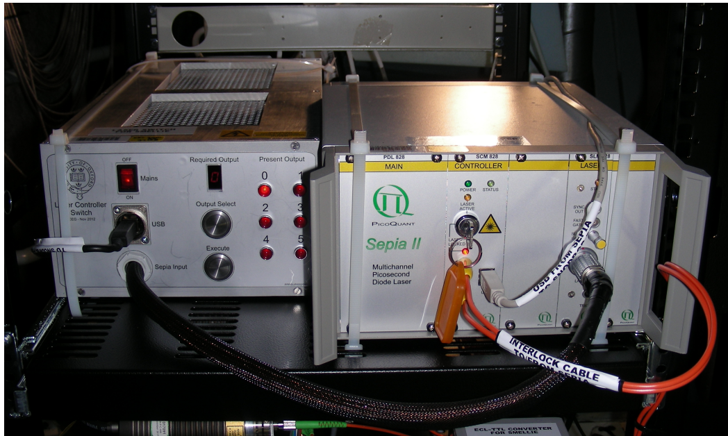
Figure 4.7: The Laser Switch (left) and the SEPIA II Laser Driver (right) connected by a LEMO cable (black). The Laser Switch's output sockets are located on the rear of the device. Also shown are the laser head interlock key and cables (orange) on SEPIA, the front panel controls on the Laser Switch, and the USB connections between the SMELLIE Control PC and each component.
