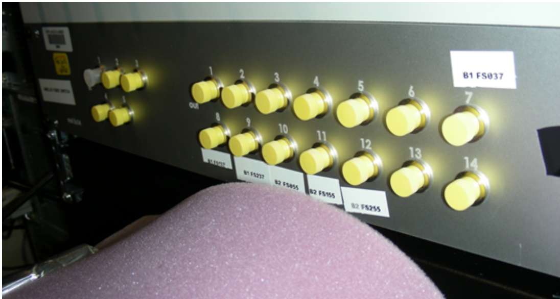
Figure 4.9: The front panel of the Fibre Switch, with the 5 input fibre sockets on the left and the 14 output sockets on the right. At the time of this picture, the detector fibres were not connected to their respective output sockets, but instead were temporarily housed under the pink foam in the foreground. The RS232 socket that connects the Fibre Switch to the SMELLIE Control PC is located on the rear.
