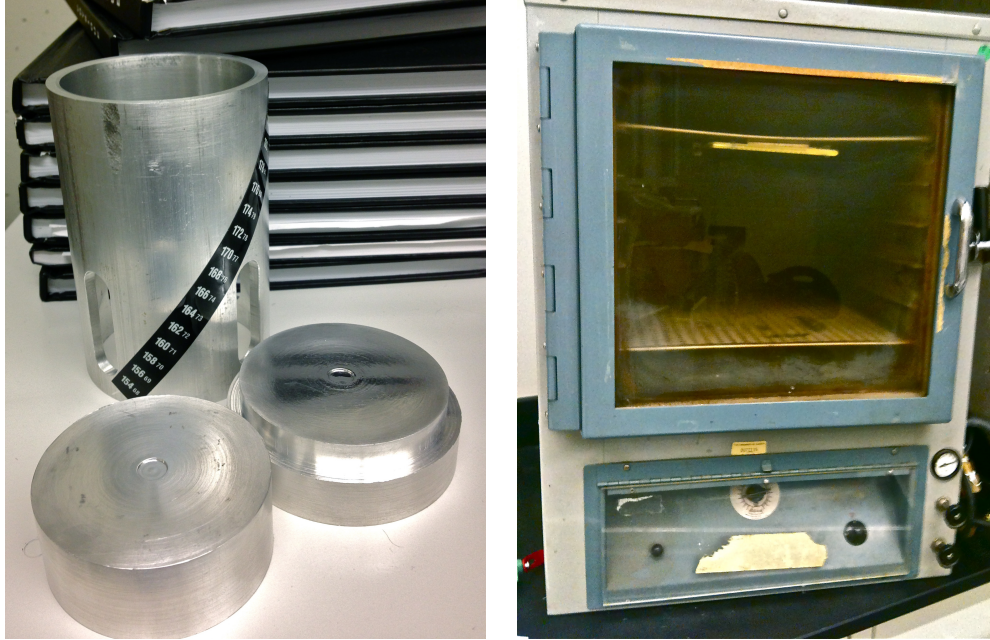
Figure 4.3: I constructed an aluminum bonding jig (left) to hold the scintillator buttons in the oven (right) during the heat-sealing process.
