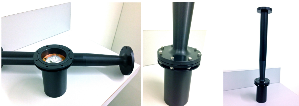
Figure 4.17: The Delrin ® encapsulation consists of a container with 2 mm thick walls that houses the copper encapsulation (left). Eight screws connect this container to a stem at a flange (middle), which compresses an internal o-ring to provide a leak-tight seal. When connected (right), the Delrin ® layer is nearly 398 mm in height. This does not include the source connector that will attach to the top of the stem.
