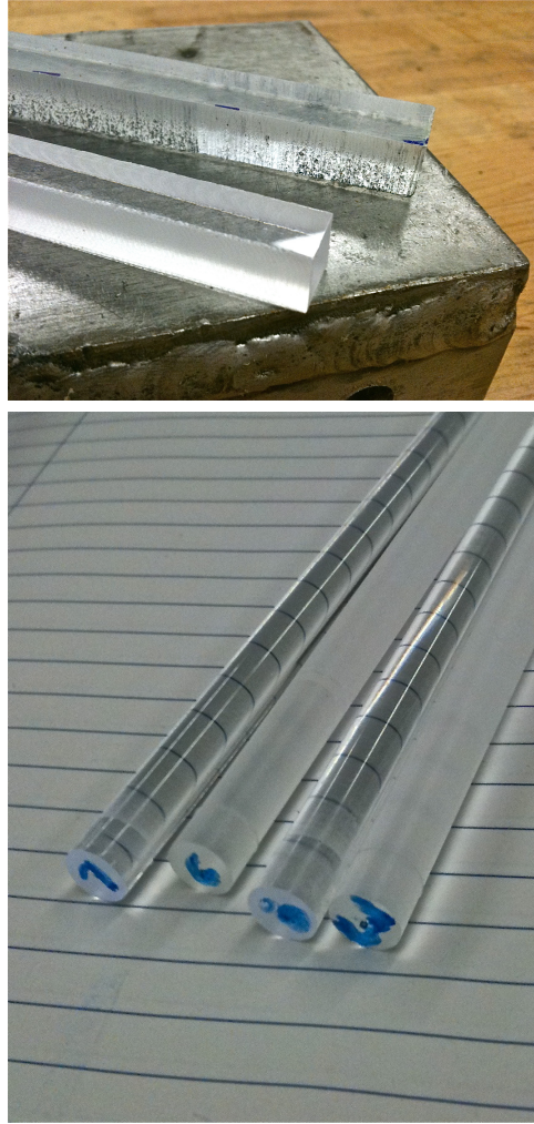
Figure 4.1: Rough-cutting the plastic scintillator resulted in significant marking of the cut sides (top). After turning on the lathe, the scintillator cylinders had a somewhat rough surface finish (cylinders 6 and 3), which the polishing process made clear (cylinders 7 and 8) (bottom).
