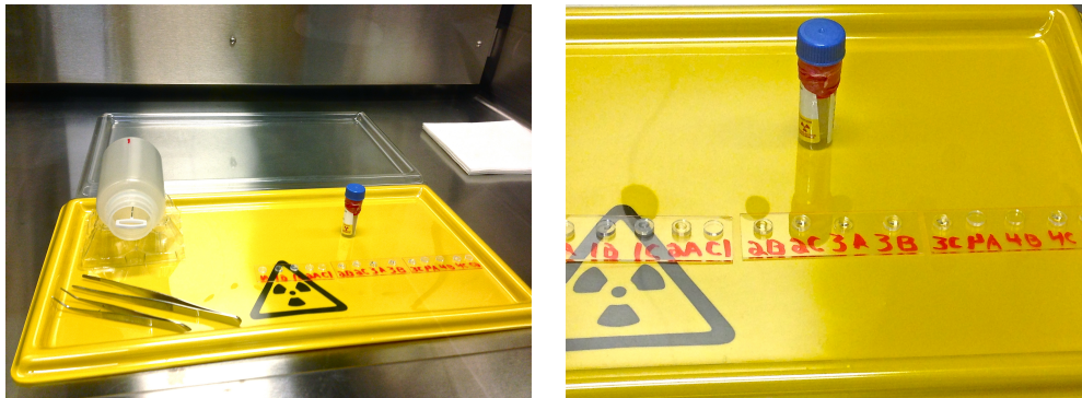
Figure 4.2: I deposited the liquid ^{60}\text{CoCl}_2 \cdot 6\text{H}_2\text{O} onto the buttons in a fume hood, set up as shown (left). The liquid collected at the centre of each button (right). The size of the liquid drop depended on the number of droplets required to obtain the necessary activity.
