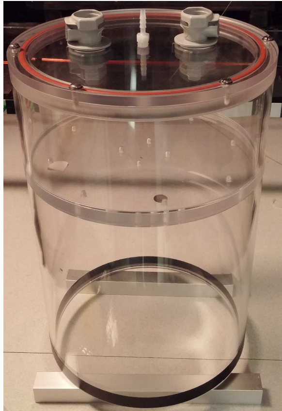
Figure 6.6: Scout inner vessel and stand, constructed in the UC Davis machine shop.
