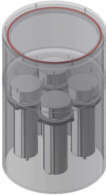
Figure 6.5: CAD drawing of the Scout detector with the PMT support rings shown compressing the PMTs into the bottom of the acrylic vessel.
