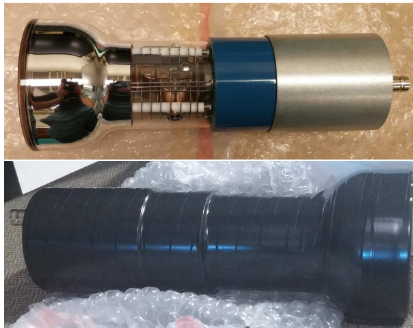
Figure 6.7: ADIT 3-inch photomultiplier tube with connected base. Top shows the PMT dynodes through the glass, and bottom is the PMT wrapped in electrical tape to prevent light from entering and exiting the sides.
