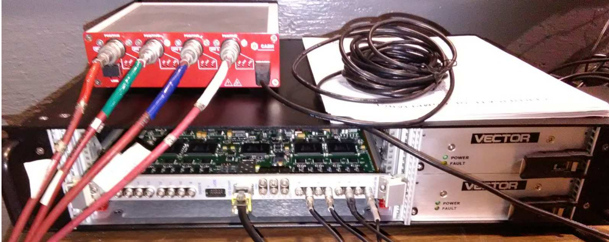
Figure 6.8: Scout data acquisition system with 4 channels with independent high voltage settings (red box) and a VME powered 16 channel waveform digitizer.
