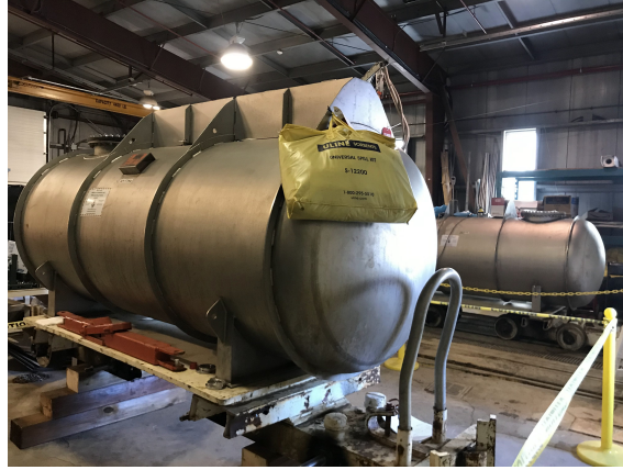
Figure 3.5: A photo of the two tonne rail cart used for scintillator transfers.
