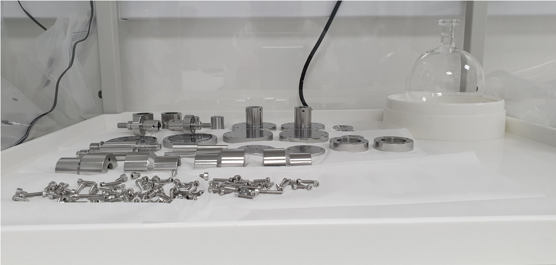
Figure 3.12: Cleaning of the laserball sphere and corresponding parts in the clean room at the University of Sussex.
