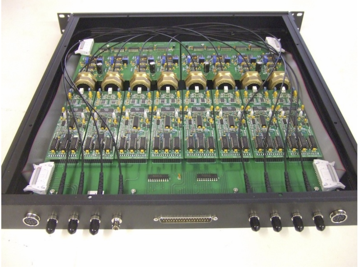
Figure 7.2: The internals of a TELLIE driver box. The eight small boards at the bottom of the image are the LED driver boards. The LEDs and the PIN diodes are encased in the brass fittings shown in the center of the image. The two larger boards at the top of the image are the PIN diode monitoring boards.
