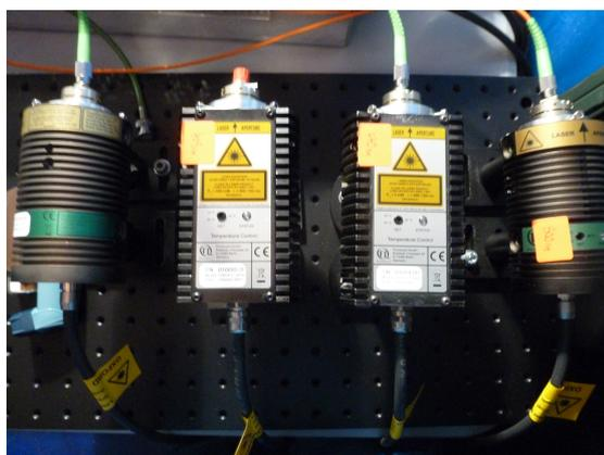
**Figure 4.3:** The four SMELLIE single-wavelength laser heads.
