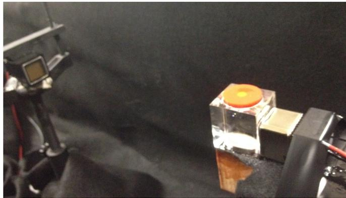
**Figure 7.12:** The scintillator emission timing setup, which includes an R7600-U200 PMT optically coupled to the scintillation source, which is used as a fast trigger. In this picture, a red  $^{210}\text{Po}$  disk source is deployed above a sample of liquid scintillator, held inside a UVT acrylic block. A second R7600-U200 PMT located about 30 cm away from the scintillation source.
