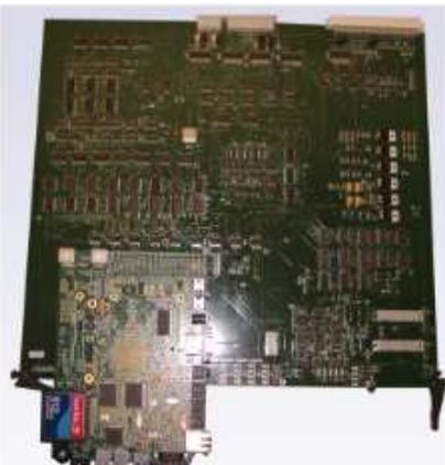
(b) The XL3 read out board, developed primarily by R. Bonventre.
