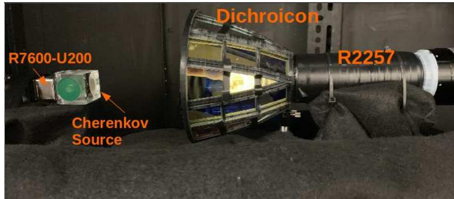
**Figure 8.27:** A side view of the dark-box setup with the Cherenkov source. The dichroicon is shown with the R2257 PMT at the aperture. In front of the R2257 PMT is a 480 nm longpass dichroic filter. The barrel of the dichroicon consists of shortpass dichroic filters. The reflecting cylinder and R1408 PMT are not shown in this setup. The distances and size of the various important components is shown in Figure 8.26.
