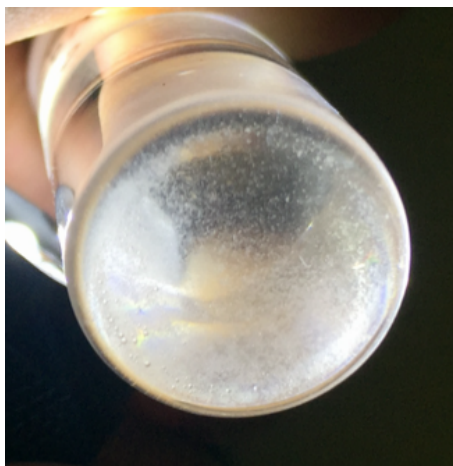
Figure B.1: Photo of precipitation formed in a sample with tetradecylamine after humidity exposure.
