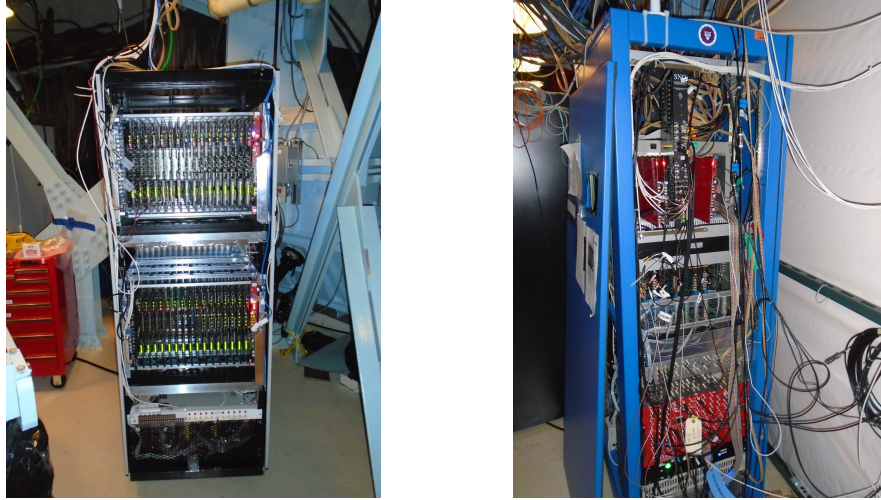
Figure 3.6: Images of a SNO+ rack holding two crates (left) and the central electronics rack (right).
