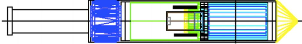
Figure 2.7: The  $^{16}\text{N}$  source as implemented in the SNO+ simulation package. The blue box to the right represents the decay chamber. It is observed by a scintillation chamber (green) which also holds a PMT (black). Figure is from [48].
