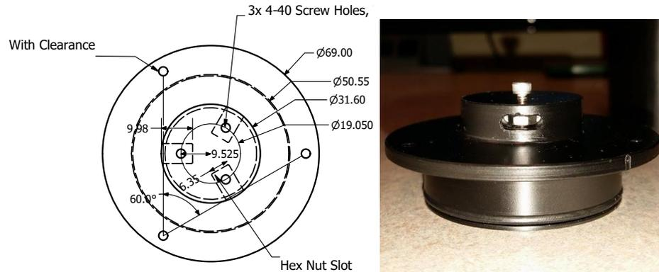
Figure 3.5: The “captured nut” structure. Figure to the left is from [56].
