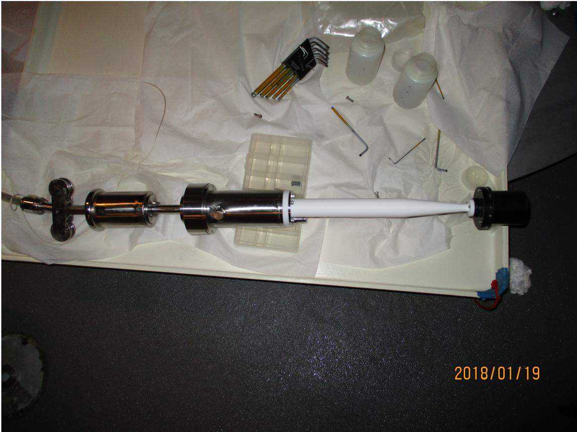
Figure 3.7: The  $^{241}\text{Am}^9\text{Be}$  source assembly was attached to the stem and carriage. The umbilical and central rope were still mounted on the URM, but can be seen to the left side of the figure.
